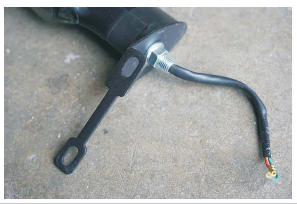
5. Attach the turn signal harness extension kit to the left/right signal output. The extension kit will aid in wire management due to the obstruction of the cross plate on the Grom's sub frame.
