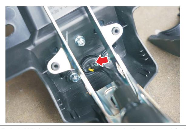
3. Unplug the left/right signal bullet connectors and unbolt signals (1 large nut for each signal), there is metal spacer that will come out which will no longer be used. Continue to completely remove the harness assembly and plug it back into the bike.
