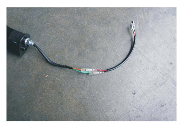
6. Mount the signal assembly behind the plate holder to the same holes for the license plate using four M6x16mm bolts, M6 large OD washers and M6 lock nuts. Bolt>License Plate>Plate Holder>Signal Bracket>Washer>Nut. Feed the signal wires through the opening on the plate holder and plug back into the harness from step 3.
